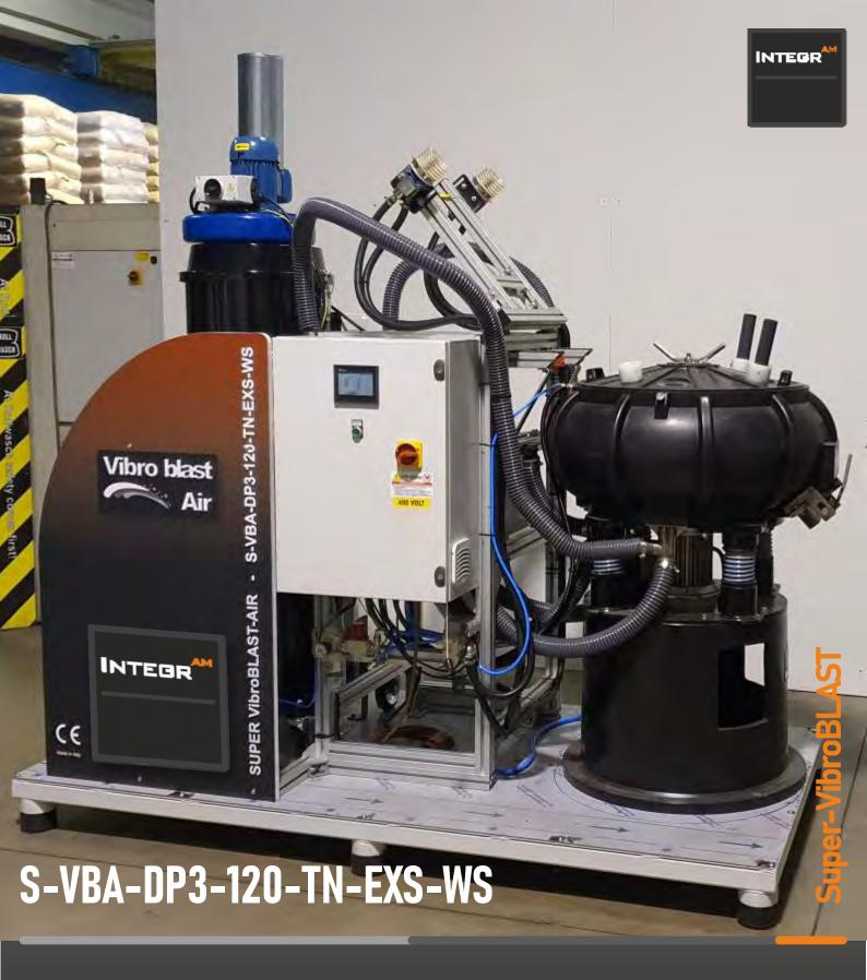
The Super VibroBLAST Air DP line is designed and manufactured to be supplied on a technological pallet, to make its installation immediate through a simple plug-&-play operation.
