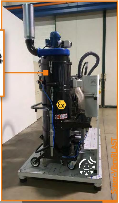
All Super VibroBLAST Air DP systems have been designed to ensure excellent aspiration and filtration, with ATEX Zone level 20 or 22 inside the aspiration unit.
