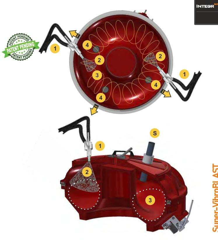
All Super VibroBLAST Air DP systems have TN (Top Nozzle) sandblasting nozzles placed in the cover upper area, to involve from above the treated components, while they rotate three-dimensionally, clockwise, inside the circular vibro-blasting tank.
