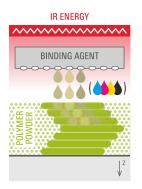
Tiny liquid droplets are applied
