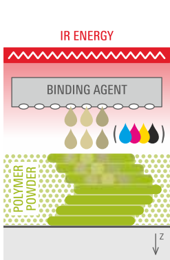
Tiny liquid droplets are applied locally to a layer of polymer powder. They increase or suppress the heat absorption of the powder. An integrally acting infrared source melts the material respectively.
