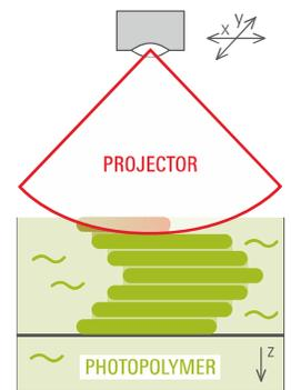
A photopolymer is exposed layer by layer using a projector. The exposed material is polymerized locally and solidifies.
